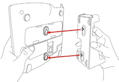
To attach the Mounting Bracket (MB), align the two cleats on the MB with the holes in the phone's base.
