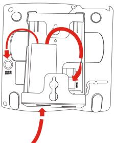
Plug in the Ethernet and power cables.
