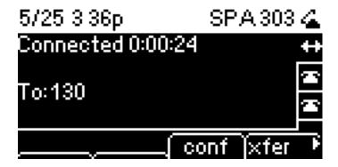
In the figure above, the double arrow on the right of the screen indicates that a call is in progress. The offhook phone icon next to "SPA 303" indicates the handset is in use.
