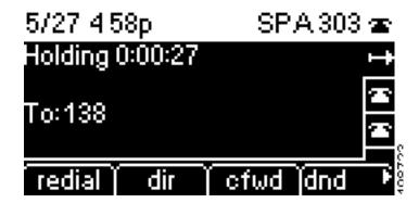
In the figure above, the right arrow on the right of the screen indicates that a call is on hold.
