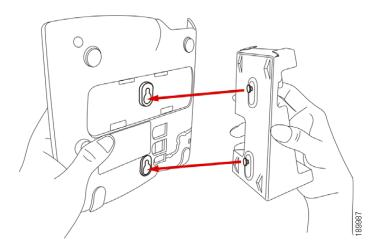
STEP 2 Orient the MB such that the phone's Ethernet and handset ports are accessible after installation.
