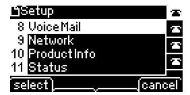
The IP address is displayed on the Network screen.
