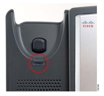
Figure 5 Handset Retention Tab (Default Position)
