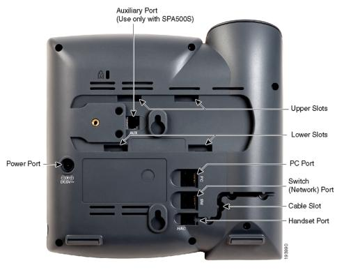
**STEP 1** Turn the phone body over to expose the ports on the back of the unit.
