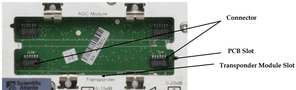
**Important Note:** Make sure that the transponder is inserted in the correct slot.
