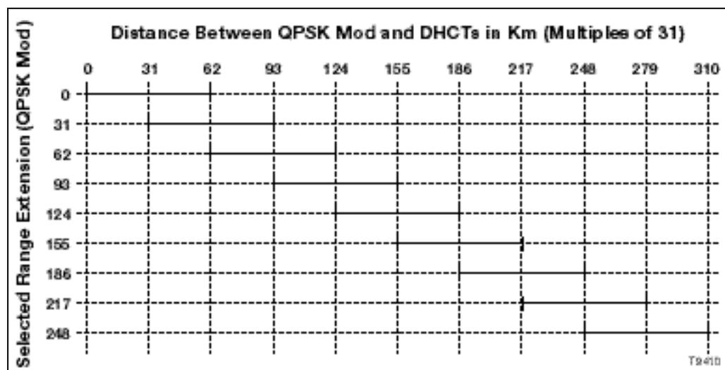
**Example:** With 155 km set on the QPSK, the closest distance you could locate a DHCT to a QPSK modulator is 155 km. The furthest distance you could locate a DHCT to a QPSK modulator is 217 km.
