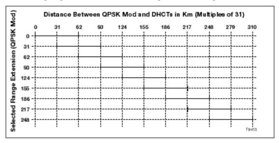
**Example:** With 155 km set on the QPSK, the closest distance you could locate a DHCT to a QPSK modulator is 155 km. The farthest distance you could locate a DHCT to a QPSK modulator is 217 km.
