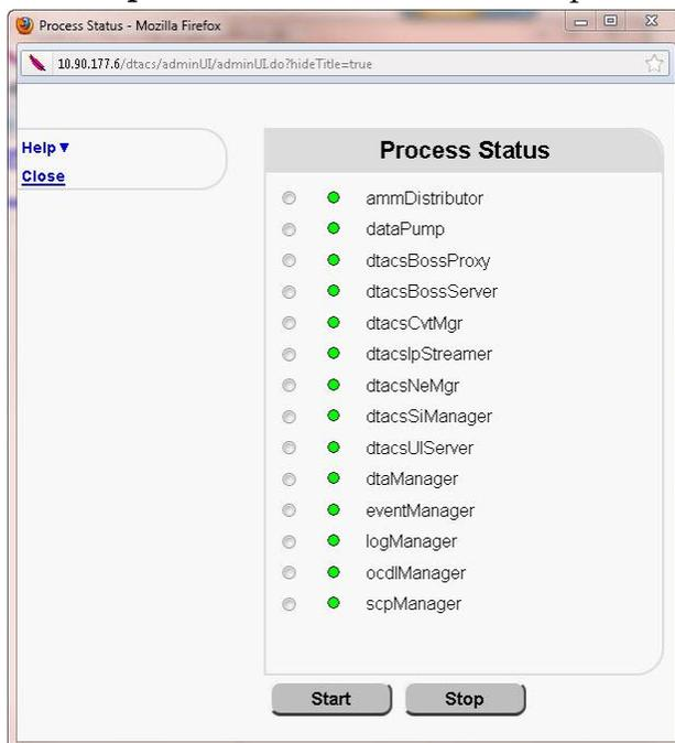
Each process running on the DTACS is listed next to a green, yellow, or red indicator. The color of the indicator shows the status of the process.
