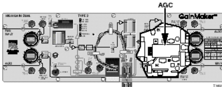
5. Replace the amplifier cover and tighten the cover screws from 10 in-lb to 12 in-lb (1.1 Nm to 1.4 Nm).
