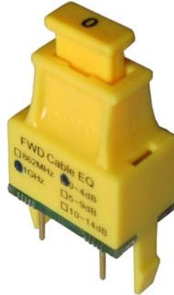
Increasing the equalizer value reduces the level at lower frequencies, relative to the level at 862 MHz / 1 GHz.
