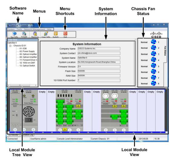
The OptoStar II console main interface shows the software name, menus, menu shortcuts, local module tree view, system information, chassis fan status, and local module view.
