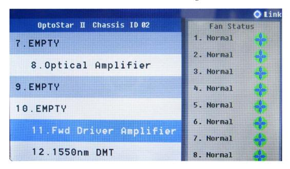
Press ▼ button to move the cursor down to Fwd Driver Amplifier (OptoStar II forward driver amplifier module), and press the SET button to enter the sub-menu of the forward driver amplifier module.
