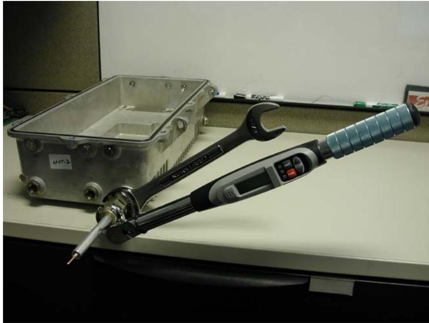
This photo illustrates the recommended method for tightening the back nut. The torque wrench is fitted with a flare nut crow's foot, shown in detail below.
