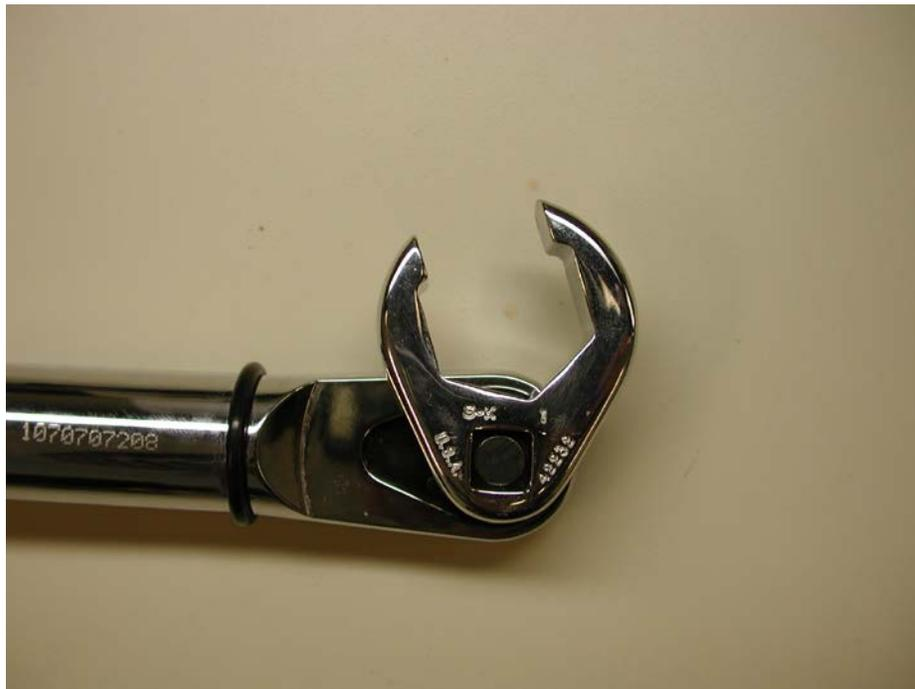
This accessory offers the benefit of capturing the nut so that the wrench will not slip off, an especially helpful feature when working from a bucket truck.
