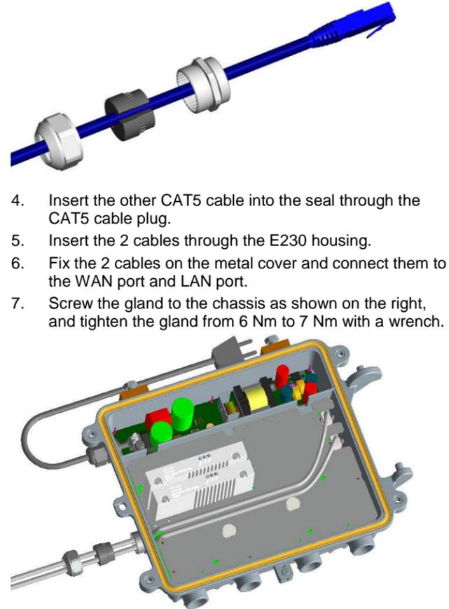
4. Insert the other CAT5 cable into the seal through the CAT5 cable plug.
