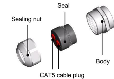
3. Insert the CAT5 cables into the seal through the CAT5 cable plug.
