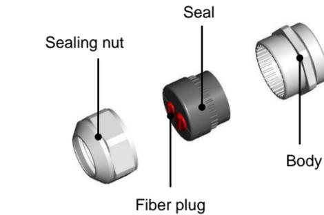
3. Insert the fiber into the seal through the fiber plug.
