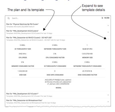
Workload Optimization Manager runs nightly plans to calculate headroom for the clusters in your on-prem environment. For each cluster plan, you can set which VM template to use in these calculations.
