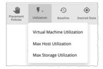
Max Host Utilization levels specify the percentage of the physical resource that you want to make available in the given plan. By default, hosts have utilization set to 100%. For a given plan, you can set the utilization to a lower value. For example, assume you want to simulate High Availability of 25% for some hosts in the plan. In that case, you can select these hosts and set their utilization levels to 75%.
