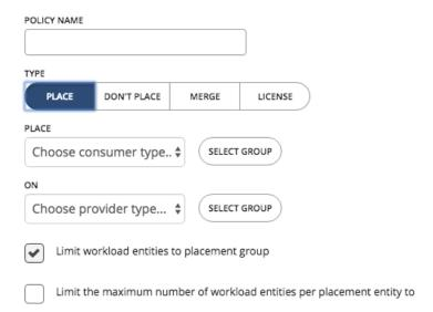
These policies control where workload can be placed. For example, you can specify that a VM will only be placed on a host that is a member of a specific cluster. Or you could specify that any applications in a specific group can only be placed on a datastore that is a member of a specific group.
