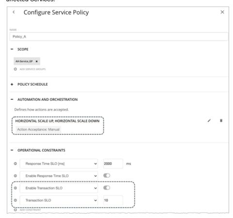
Transaction SLO is the maximum number of transactions per second that each Application Component replica can handle.
