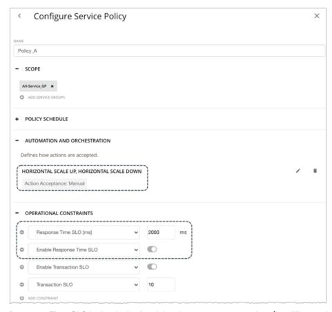
Response Time SLO is the desired weighted average response time (in milliseconds) of all Application Component replicas associated with a Service.
