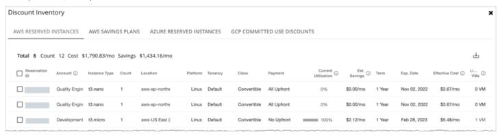
Each row in the table corresponds to a discount. Note that there can be several discounts for an Azure subscription or AWS/GCP account, and each discount displays as its own row. Table columns show basic information obtained from the cloud provider, such as the name/ID of the discount, the subscription/account that uses that discount, instance type and location, term, and expiration dates. Click a subscription/account to narrow the scope.
