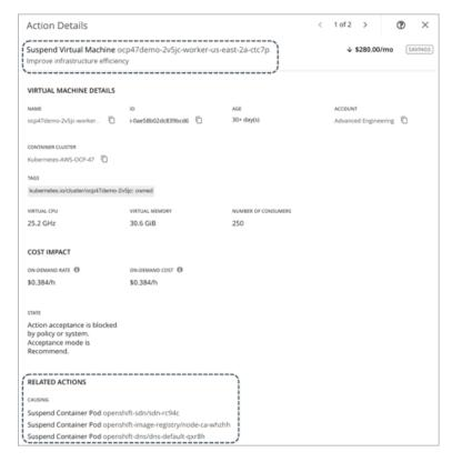
Workload Optimization Manager treats static pods as DaemonSets for the purpose of suspending nodes. Because a static pod provides a node with a specific capability, it is controlled by the node and is not accessible through the API server. If the only workload type left on a node is a static pod, Workload Optimization Manager generates actions to suspend the node and the corresponding static pod.
