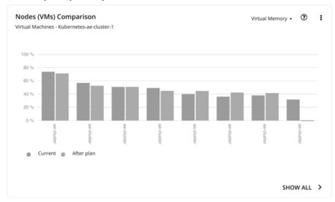
This chart compares node resource utilization (one metric at a time) before and after the plan.
