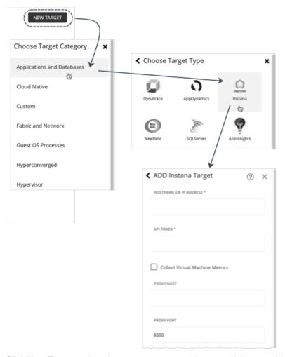
Click New Target, select the target category and type, and then provide the address and credentials for that target.
