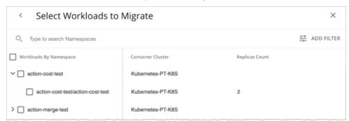
Container workloads are grouped by namespace. Expand a namespace to see individual Workload Controllers that manage workloads, and the number of container replicas for each Workload Controller. You can adjust the number of replicas in a later step. For example, you can add replicas to meet workload demand.
