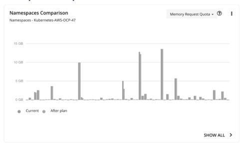
This chart compares namespace quota usage (one metric at a time) before and after the plan.
