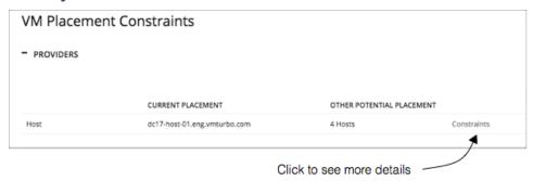
When you drill down to a single entity, you can see details about the entity's relationships in the supply chain. This shows you which entities provide resources to this entity. When considering providers for this entity, you can see the name of each current
