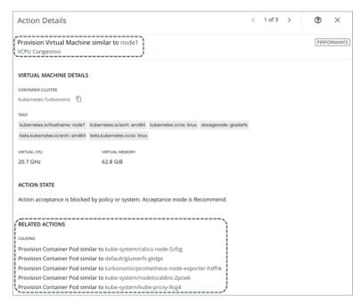
Workload Optimization Manager treats <u>static pods</u> as DaemonSets for the purpose of provisioning nodes. Because a static pod provides a node with a specific capability, it is controlled by the node and is not accessible through the API server. If a node to be provisioned requires a static pod, Workload Optimization Manager generates actions to provision the node and the corresponding static pod.
