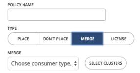
You can create placement policies that merge multiple clusters into a single logical group for the purpose of workload placement.
