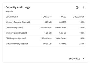
For a namespace that does not have defined quotas, *Capacity* for the commodity is infinite (as shown in the image below). *Used* values are the sum of resource limits and/or requests set for all pods in the namespace. If these are not set, *Used* value is 0 (zero).
