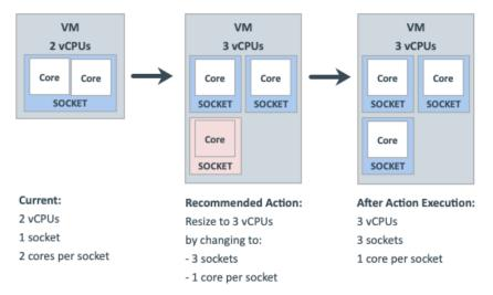
■ When the same VM needs to reduce compute capacity by 1 vCPU (i.e., from 3 to 2 vCPUs), a resize down action changes sockets from 3 to 2.
