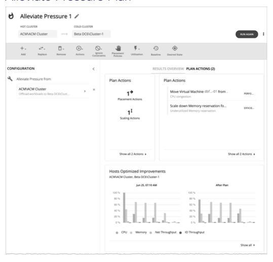
Use the Alleviate Pressure plan to find out how to migrate workloads from a stressed or *hot* cluster over to a cluster with more headroom. This plan shows the minimal changes you need to make to reduce risks on the hot cluster.
