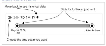
You can set a time frame from recent hours to the past year, and set that to the charts in the view. Use the Time Slider to set specific start and end times within that range. The green section in the slider shows that you can set the time range to include a projection into the future. For this part of the time range, charts show the results you would see after you execute the current set of pending actions.
