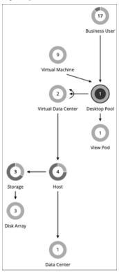
The desktop pool gets compute and storage resources from the underlying Virtual Datacenter. For VMware Horizon View, the VDI architecture includes one or more vCenter Server instances. When it discovers the Horizon View target, Workload Optimization Manager also discovers the supporting vCenter Server instances, and their corresponding Virtual Datacenters. These are the source of compute and storage resources for the associated desktop pools.
