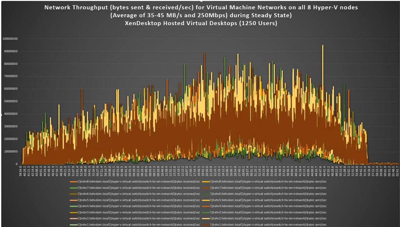
Figure 120 HyperFlex Cluster UI Performance Chart for Knowledge Worker Workload Running 1250 User Test on Citrix PVS Non-persistent Windows 10
