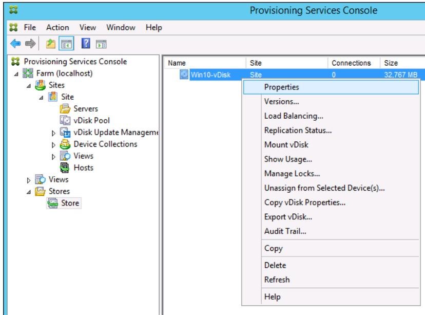
30. On the vDisk Properties dialog, change Access mode to “Standard Image (multi-device, read-only access)”.
