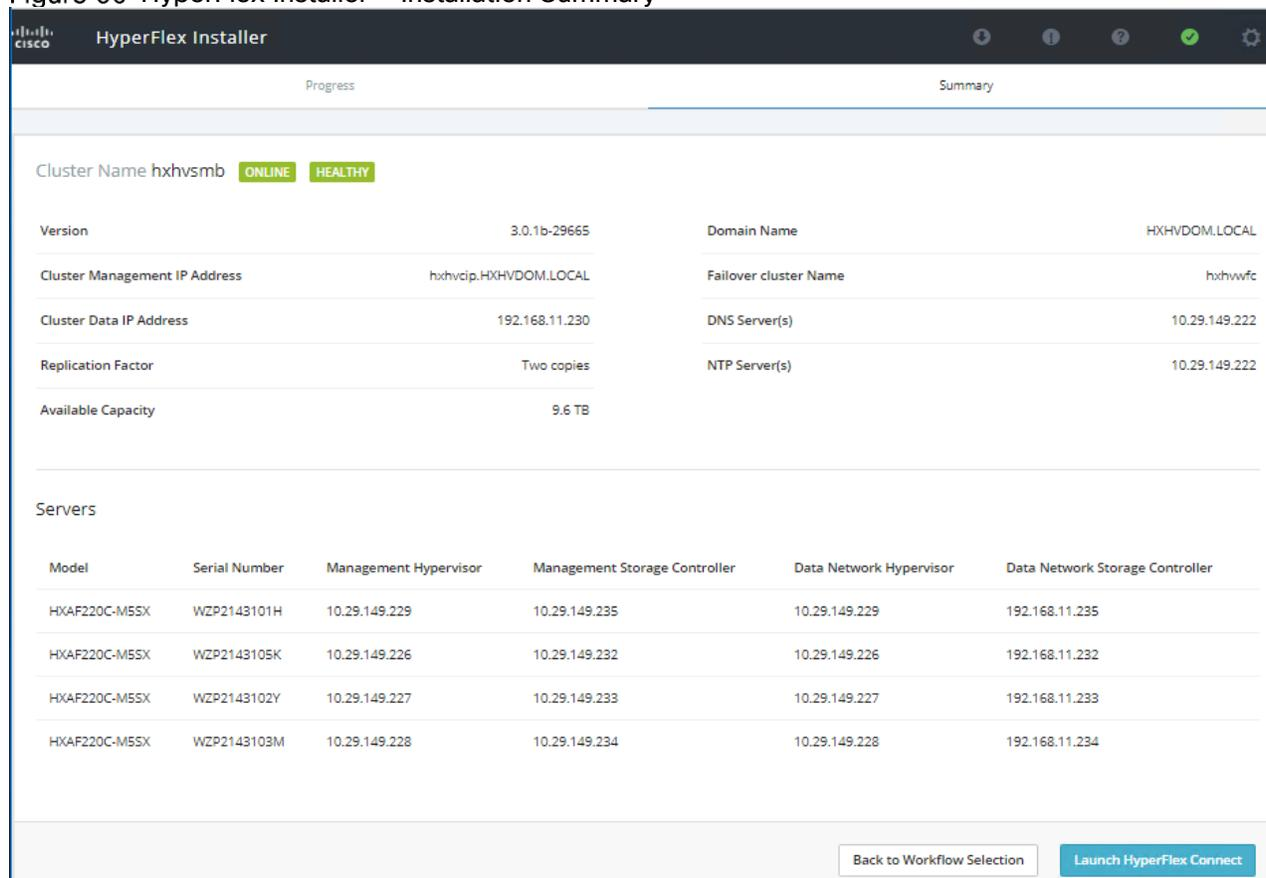
20. After the install completes, you may export the cluster configuration by clicking the downward arrow icon in the top right of the screen. Click OK to save the configuration to a JSON file. This file can be imported to save time if you need to rebuild the same cluster in the future, and stored as a record of the configuration options and settings used during the installation.
