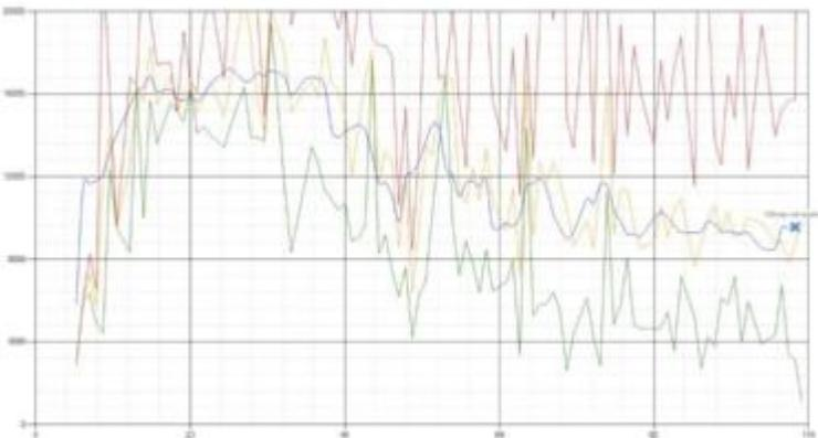
When the test is finished, VSI<sub>max</sub> can be calculated. When the system is not saturated, and it could complete the full test without exceeding the average response time latency threshold, VSI<sub>max</sub> is not reached and the amount of sessions ran successfully.
