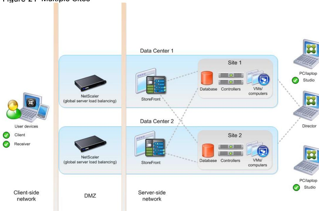
You can use StoreFront to aggregate resources from multiple sites to provide users with a single point of access with NetScaler. A separate Studio console is required to manage each site; sites cannot be managed as a single entity. You can use Director to support users across sites.
