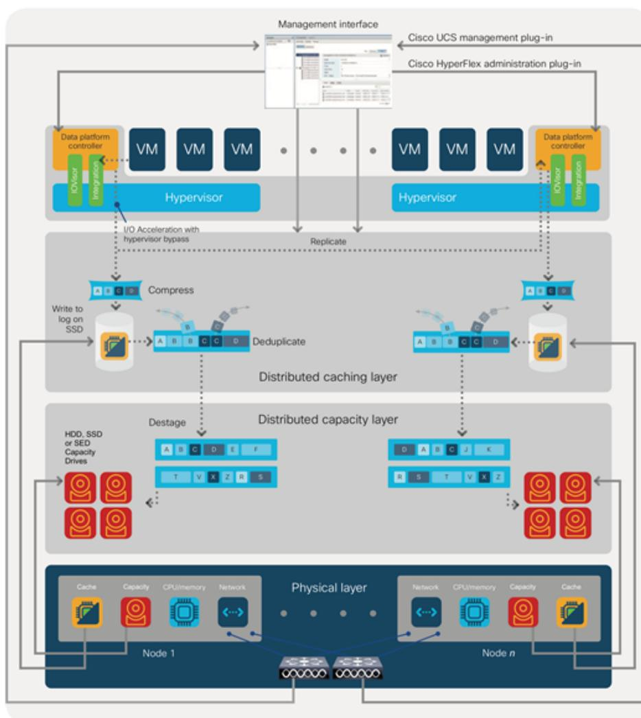
Hot data sets, data that are frequently or recently read from the capacity tier, are cached in memory. All-Flash configurations, however, does not use an SSD read cache since there is no performance benefit of such a cache; the persistent data copy already resides on high-performance SSDs. In these configurations, a read cache implemented with SSDs could become a bottleneck and prevent the system from using the aggregate bandwidth of the entire set of SSDs.
