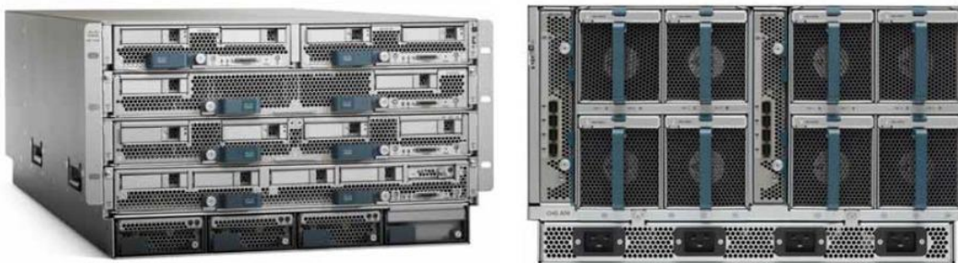
Figure 21 Cisco UCS 5108 Blade Chassis Front and Rear Views
