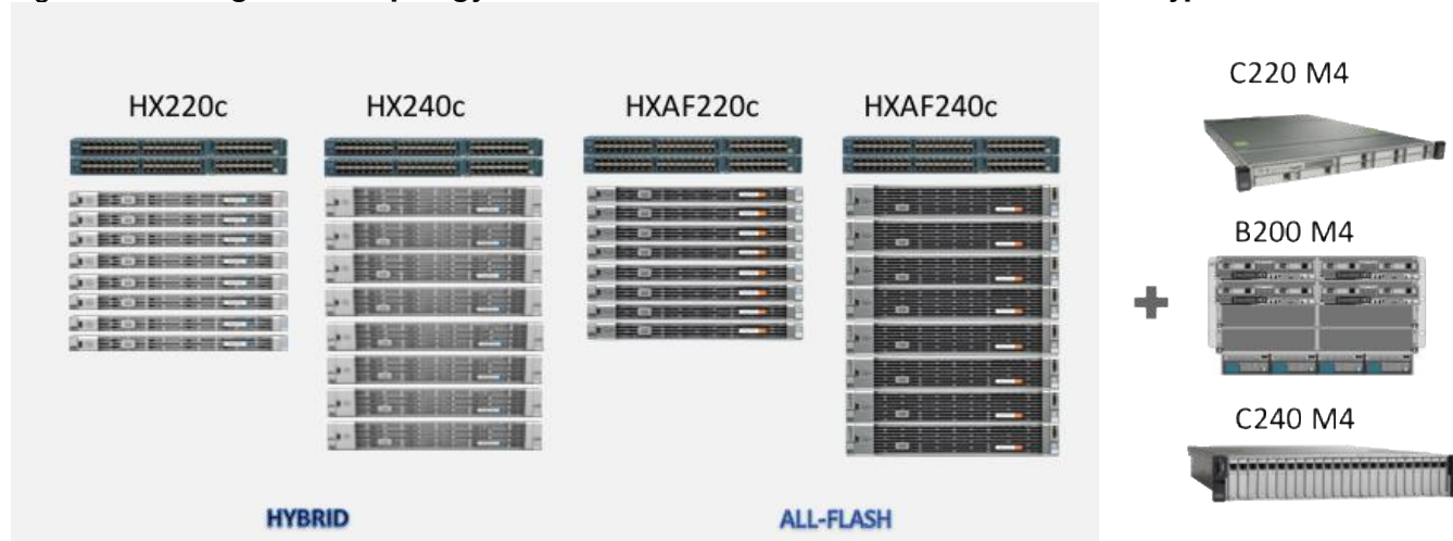
Figure 45 Configuration Topology for Scalable VMware Horizon 7 Workload with HyperFlex
