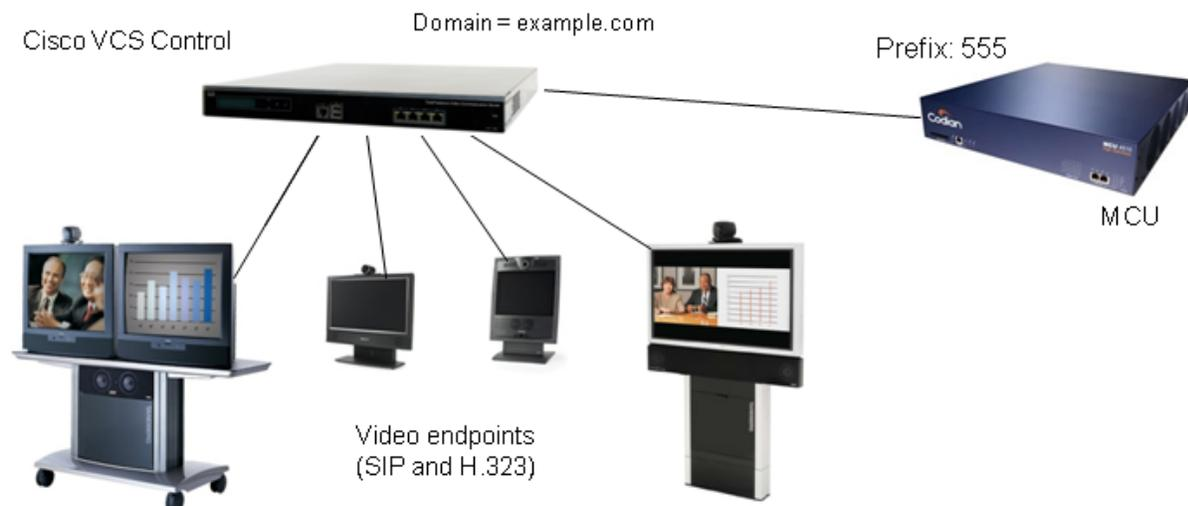
In this scenario, the MCU will be set up to receive calls with a prefix 555.
