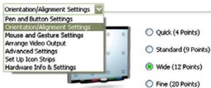
4. Press ORIENT to display a 12-touch point test pattern. Touch the center of each crosshair on the image displayed on the whiteboard. With Synch connected between the interactive whiteboard and the computer, press the \* button quickly on the remote 5 times. The on-screen message "CALIBRATION MODE" will appear. On the C-Series Codec, you will see a DIAL SCREEN appear -- ignore this and press the HOME key on the remote until the menus clear.
