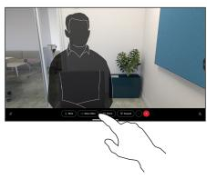
Connect your source with a cable, and make sure it's switched on. Tap the screen to get the call controls and then tap the Share button.
