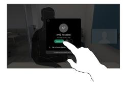
Tap the green Transfer **call** button. Talk to the person to confirm that transfer is OK. The person to be transferred is still on hold.
