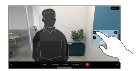
Make sure your camera is on. During a call, tap the screen to open the selfview up on top of the call. Then tap the button on the selfview's right corner and change the visibility to Hide, Show in call, or Always show.
