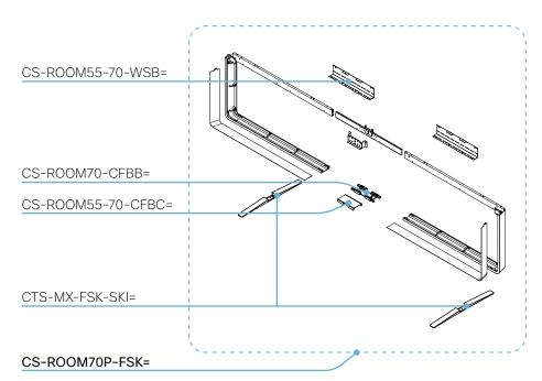
For Room 70 Panorama with the **content screen below** the main screens. This stand is higher than the other stand. For ergonomic reasons, we don't recommend using this stand for systems with a 65" content screen above the main screens, even if the ceiling height should allow for it.
