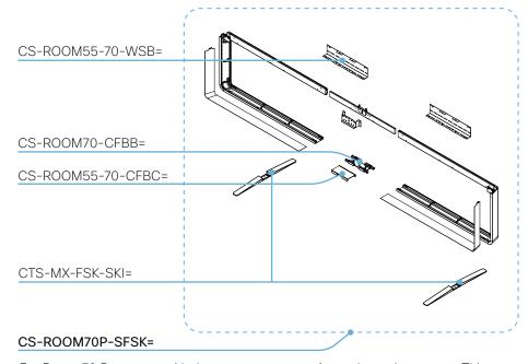
For Room 70 Panorama with the **content screen above** the main screens. This stand is lower than the other stand, and cannot be used with the 55" content screen below the main screens.
