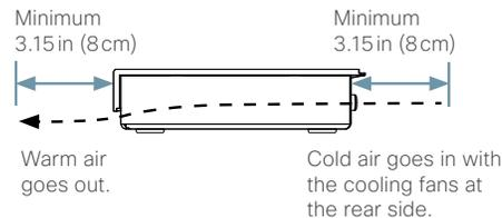
**WARNING:** If the Codec C20 is mounted with the front side or rear side down, make sure there is sufficient free space to allow for ventilation.
