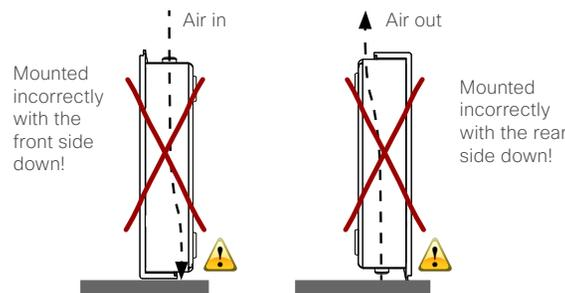
**NOTE:** Incorrect mounting as shown above will not allow for enough ventilation through the codec.
