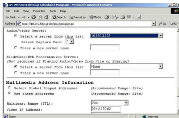
Scroll further down until you see 'Multimedia Address Information'. Select 'Use These Addresses' and enter the Multicast addresses as defined in the streaming settings on the codec for both video and audio. The port number for the video shall be the same as the 'Address port setting' on the streaming settings on the codec, while the audio port number is 4 more than the Video port.
