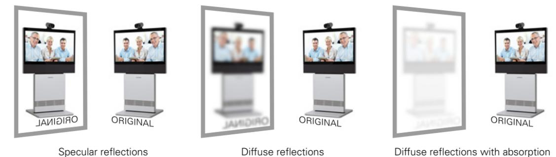
**Above:** Sound reflected off a wall resembles very much reflections of light. Specular reflections, as shown to the left, are similar to reflections seen in a regular mirror, while diffuse reflections, as shown in the middle, resembles a blurring mirror. Diffuse reflections *with* absorption provides a blurred “washed-out” reflection as shown to the right.
