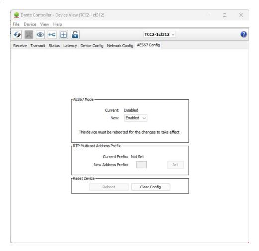
Reboot the device in the Sennheiser Control Cockpit. When the device is back up, click the button to create a new multicast flow.
