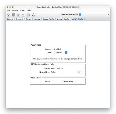
Reboot the microphone. When it is back up, click the button to create a new multicast flow.
