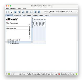
Double click the microphone's name to access its settings. First enable AES67 under the "AES67 Config" tab.
