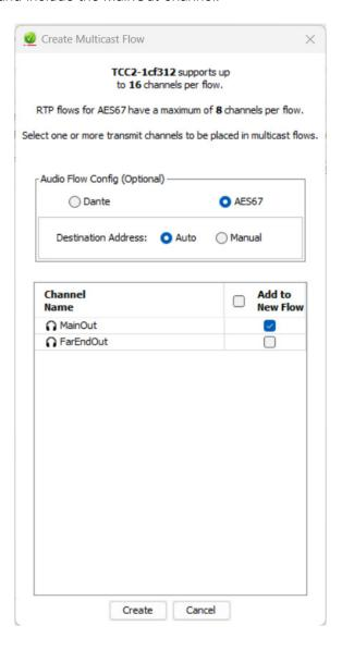
Dante automatically chose the name TCC2-1cf312 for this microphone, and will derive stream names from this. If you want a more descriptive name, you can change it in the device config tab.
