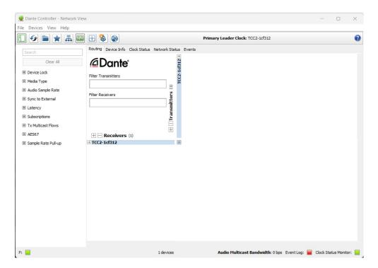
Open the device by double clicking on its name in the routing view. Now move to the *AES67 Config* tab to enable AES67 mode.
