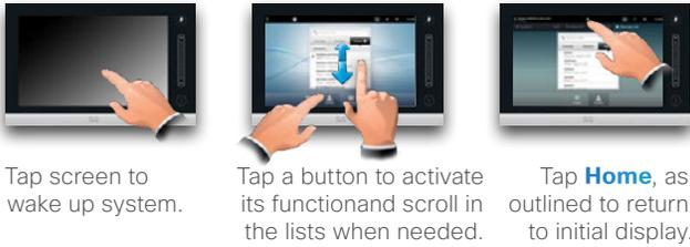
Tap screen to wake up system. Tap a button to activate its function and scroll in the lists when needed. Tap **Home**, as outlined to return to initial display.
