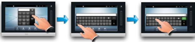
Tap **ABC**... This is the keyboard. To insert a digit tap and hold the corresponding key, or tap **123** to switch to numeric mode, as outlined. This is the keyboard in numerical mode. Tap **ABC** to go back to alpha mode.
