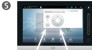
Adjust zoom in and out here. Use these controls to define the direction in which the camera shall point (also known as *Pan and Tilt* controls).
