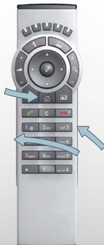
When you pick up the remote control and touch the rubber line sensors along the sides of the remote control, the system wakes up.
