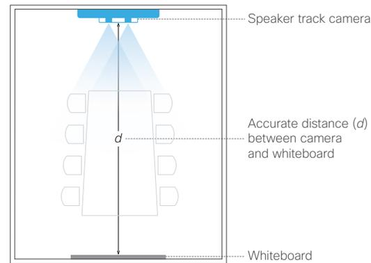
The whiteboard must be placed across the room from the camera, as shown in the illustration.
