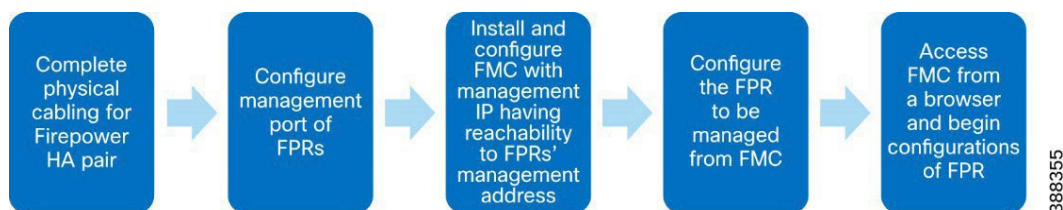
Figure 3-4: Workflow for Configuring Firepower
