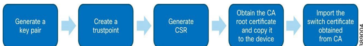
Figure 11-16 Workflow for generating certificate on a switch
