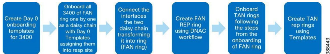
Figure 9-4: Workflow for Onboarding FAN and TAN Rings
