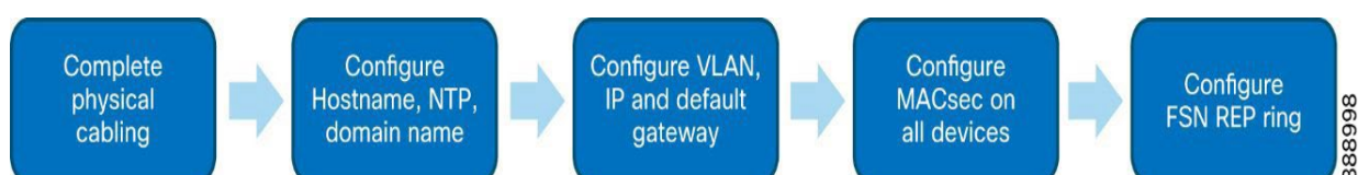
Figure 11-5 Workflow for FSN ring configuration
