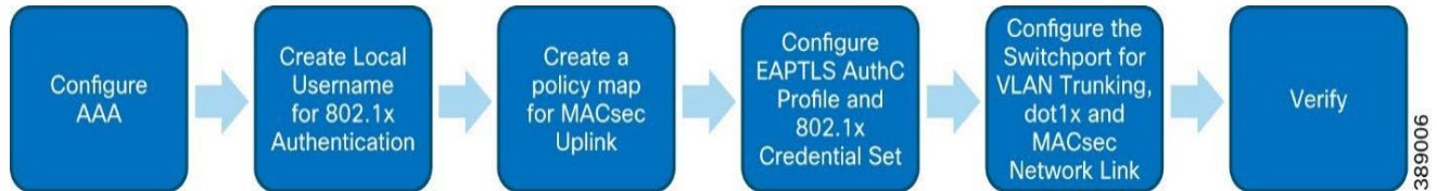
Figure 11-18 Workflow for configuring certificate based MACSec
