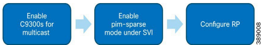
Figure 11-21 Workflow for Enabling Multicast
