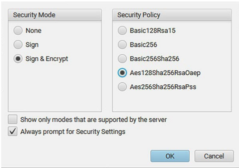
Figure 5-4: OPC-UA Client application Supporting Different Encryption Types
