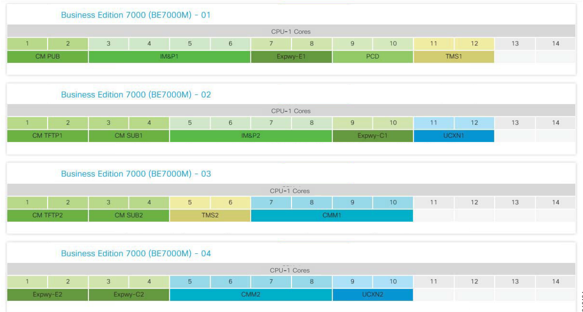
Figure 1-4 Virtual Maching Placement for Medium #1 Simplified Sizing Example
