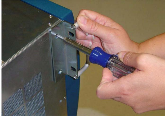
**Figure 2-1:** Remove Front or Rear Handles From Chassis, Depending on Alignment in Rack
