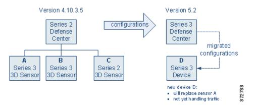
Now, you can switch the cabling from sensor A to device D to have your Version 5.2 deployment begin handling network traffic previously inspected by sensor A.
