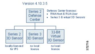
In this deployment, a Series 2 Defense Center manages three 3D Sensors deployed inline: a Series 2 sensor, a Series 3 sensor, and a 32-bit virtual sensor.
