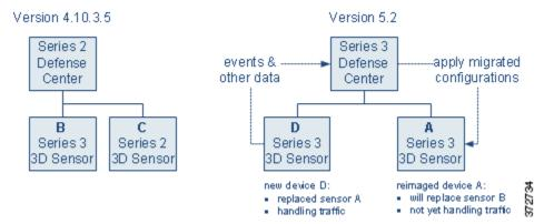
Now, you can switch the cabling from sensor B to reimaged device A to have your Version 5.2 deployment begin handling network traffic previously inspected by sensor B. Your spare sensor is now sensor B, which you can use to replace sensor C.
