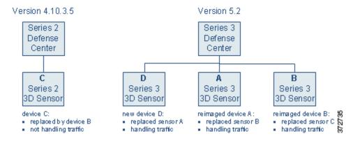
The Version 4.10.3 Defense Center is now managing only sensor C, which is not inspecting any traffic. You can power down and disconnect the sensor. However, If the Defense Center has stored events that you want to migrate, leave it powered on and connected to the management network until you perform the steps in Migrating Events from Defense Center to Defense Center, page 2-10.
