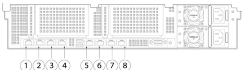
The illustration above shows a model with Ethernet ports. For models with Fiber Optic ports (S690-1G and S690-10G), call-outs 1 through 4, 7, and 8 are replaced with six Fiber Optic ports. These ports are located above the Ethernet ports shown in the illustration, and the Ethernet ports are not present. For details, see the *Cisco x90 Series Content Security Appliances Installation and Maintenance Guide*.
