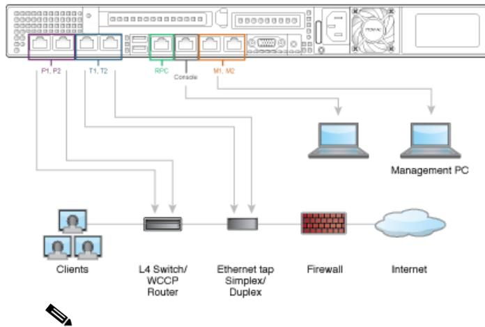
**Note** To monitor true client IP addresses, the L4 traffic monitor should always be configured inside the firewall and before NAT (Network Address Translation).
