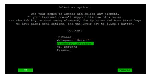
2. From the screen that opens, select the applicable Telemetry Network interface.
