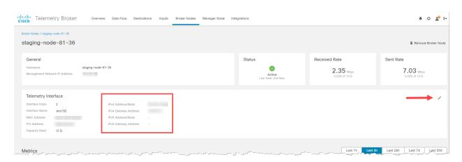
5. Configure the IP and Gateway addresses (enclosed in red border).
