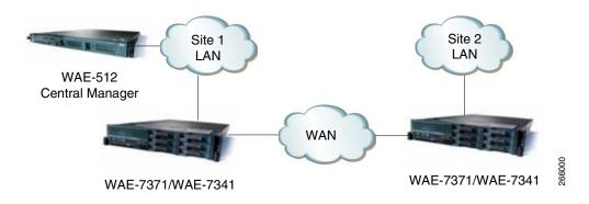
One WAE is configured in Central Manager (CM) device mode and provides a management GUI among other services. At least two additional WAEs, one in each site, examine traffic flowing through them and use built-in application policies to determine whether to optimize the traffic or allow it to pass through the network unoptimized. For high availability, a second CM device may be deployed (at Site 2 in Figure 1) as a standby.
