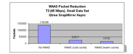
Finally, Figure 9 shows a somewhat smaller but still substantial throughput improvement for volume SnapMirror Async for data sent after a volume is deduplicated. This shows the NetApp and Cisco WAAS data redundancy algorithms are compatible.
