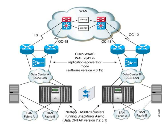
Figure 2 SnapMirror Async and Cisco WAAS Network Topology
