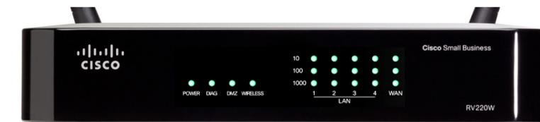
**POWER**—The Power light is green to indicate the unit is powered on. The light flashes green when the power is coming on.
