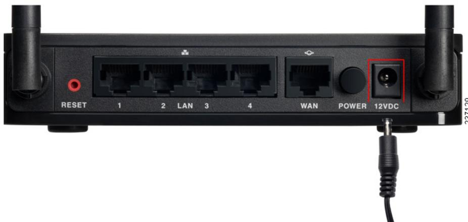
**STEP 6** Plug the other end of the adapter into an electrical outlet. You may need to use a specific plug (supplied) for your country.
