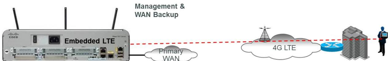
The third option combines the advantages of an ISR integrated LTE interface with an external device that provides for full redundancy of the primary ISR. The existing ISR remains in place with an 819G-4G ISR added. The 819 is a small, low cost, high function, fixed port ISR with embedded LTE and serial port.
