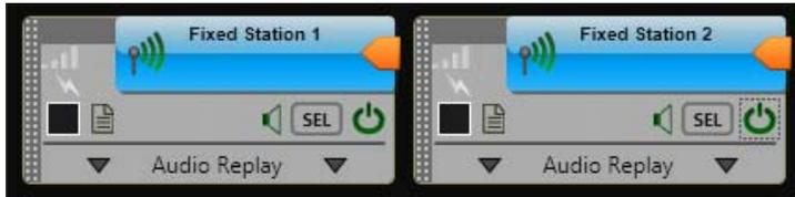
Clicking on the page icon on the talkgroup displays the details page for this fixed station. This page is used to control the fixed station.
