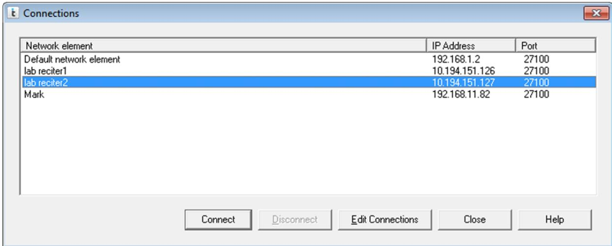
Proceed with the password prompt as previously configured. Once connected, click the “Read” icon from the toolbar. Click “Ok” if the CSS warns about overwriting a previously loaded configuration. This will load the configuration for the selected fixed station.
