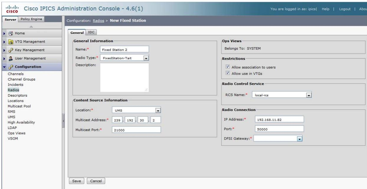
Once saved, the fixed station should have “Control Status” as CONNECTED\_ONLINE and “Functional Status” as ACTIVE.
