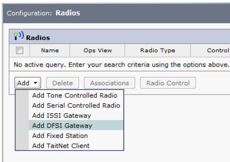
The form below allows the provisioning of a DFSIG:
