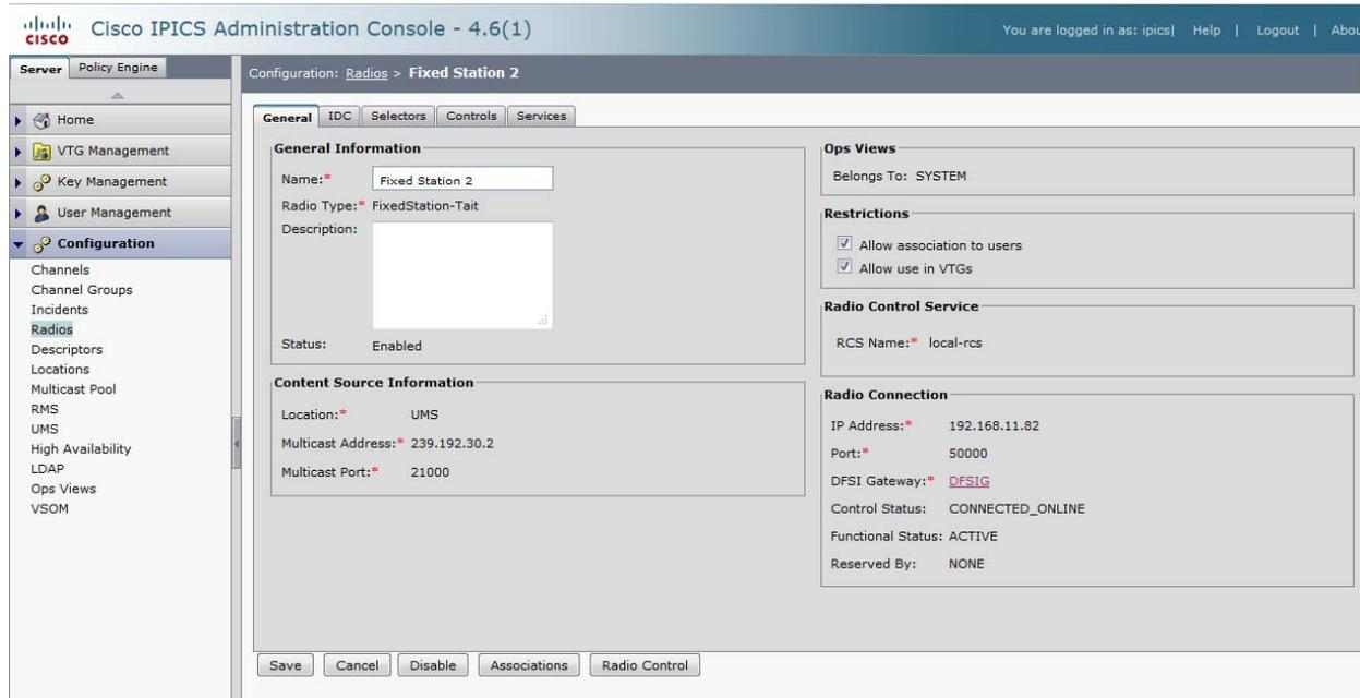
In the event the control status is something else, check the DFSIG. It means that there is a problem with the DFSIG. If the functional status is ERROR\_NO\_SERVICE, then it means that the DFSIG was not able to connect to the fixed station. This could be because the ip/port information is incorrect, a network issue or DFSI has not been enabled on the fixed station.
