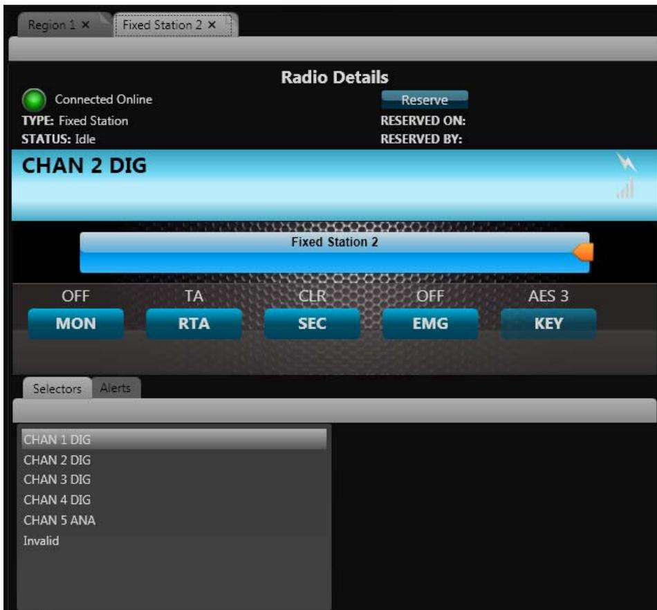
Clicking on a channel selector, causes the fixed station to switch to that channel selector. Clicking on the control functions allows the IDC user to select the state of a desired control function on the fixed station.
