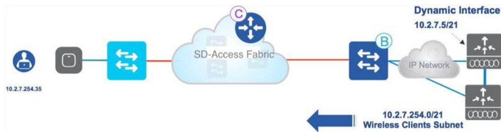
Figure 30. Wireless LAN connections
