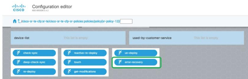
4. Set error-recovery to **sync-to**, then click **Run error-recovery action**. After successful recovery, a message is displayed.
