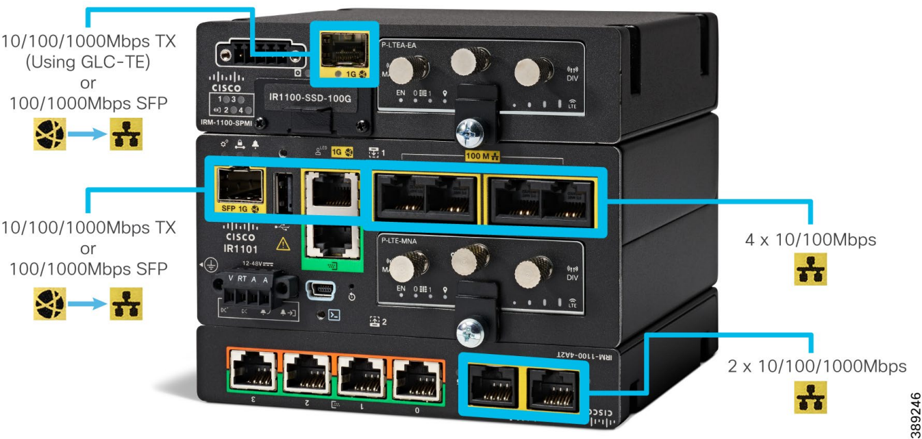
Figure 16 - IR1101 with IRM-1100-SPMI and IRM-1100-4A2T modules, and WAN ports used as LAN ports
