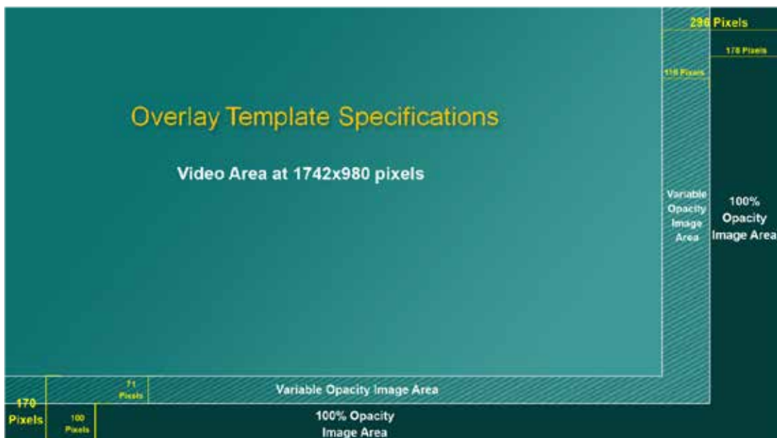
Figure 7. Overlay Template Specifications
