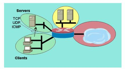
The client-servers policy is less complex than the others. Layer 4 inspection is applied from the clients zone to the servers zone. This allows connections from the clients zone to the servers zone, and allows return traffic. Layer 4 inspection carries the advantage of simplicity in the firewall configuration, in that only a few rules are required to allow most application traffic. However, Layer 4 inspection also carries two major disadvantages:
