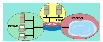
In this example, each zone holds only one interface. If an additional interface is added to the private zone, the hosts connected to the new interface in the zone can pass traffic to all hosts on the existing interface in the same zone. Additionally, the hosts' traffic to hosts in other zones is similarly affected by existing policies.
