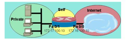
Although the router offers a default-allow policy between all zones and the self zone, if a policy is configured from any zone to the self zone, and no policy is configured from self to the router's user-configurable interface-connected zones, all router-originated traffic encounters the connected-zone to self-zone policy on its return the router and is blocked. Thus, router-originated traffic must be inspected to allow its return to the self zone.
