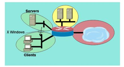
The servers-clients policy applies inspection using a user-defined service. Layer 7 inspection is applied from the servers zone to the clients zone. This allows X Windows connections to a specific port range from the servers zone to the clients zone, and allows the return traffic. X Windows is not a natively supported protocol in PAM, so a user-configured service in PAM must be defined so the ZFW can recognize and inspect the appropriate traffic.
