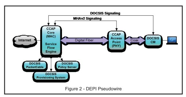
The DEPI signaling is between the CMTS (CCAP) core and the access point. The DOCSIS signaling is between the CMTS (CCAP) and the CM. In general, the Remote PHY access point is transparent to the DOCSIS signaling. One of few exceptions to this rule is that the access point has to regenerate the DOCSIS SYNC message in the downstream.
