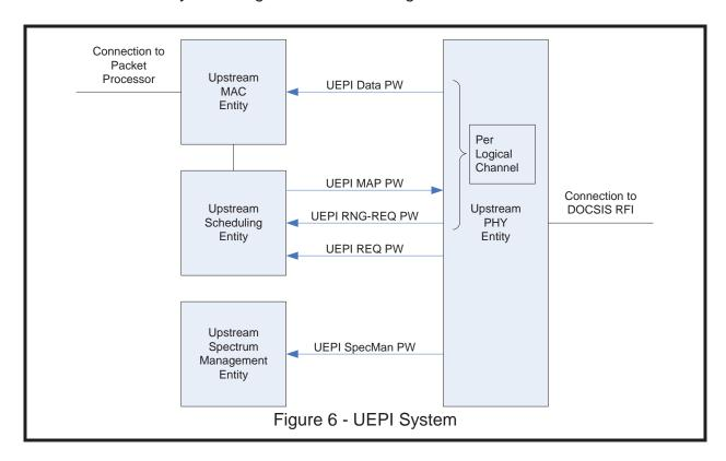
There are five pseudowires defined for UEPI. The first four are unique per QAM channel. The fifth pseudowire could be per QAM channel or per chip entity.
