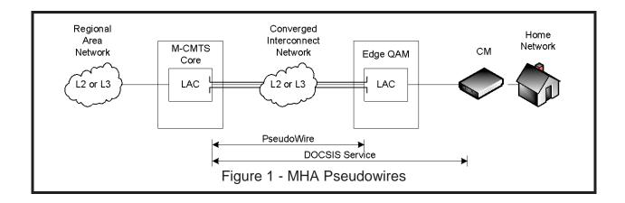
To understand DOCSIS Remote PHY, it is first necessary to understand the concept of a pseudowire (PW). A pseudowire was originally defined in "RFC 3955 Pseudo Wire Emulation Edge-to-Edge (PWE3) Architecture". The definition has evolved to:
