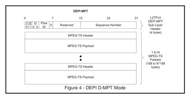
The DEPI D-MPT payload contains the exact same MPEG-TS frames that are defined in the DOCSIS specifications. In the payload of those MPEG-TS packets are the DOCSIS frames. With this format, the Remote PHY can take the MPEG-TS packets directly from the DEPI packet and map them into the SC-QAM.
