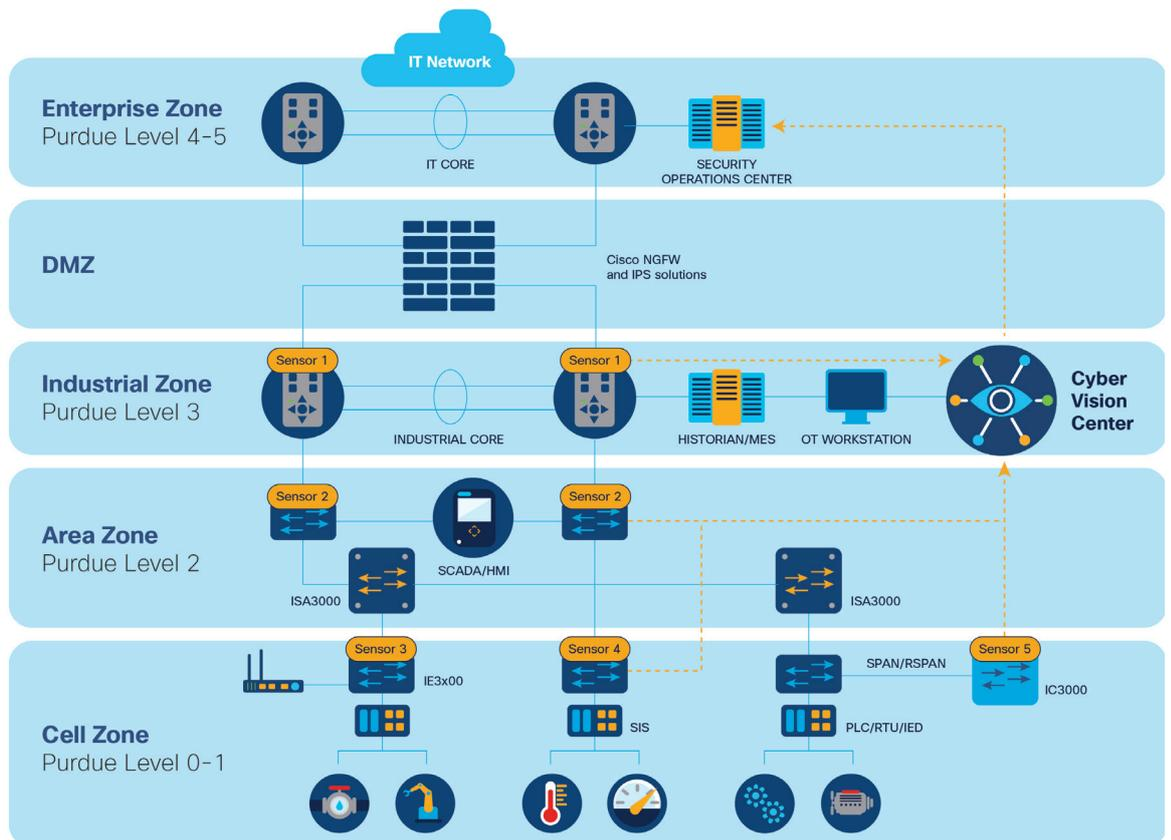
**The placement of the sensors must make it possible to monitor the different interconnection points of the industrial system:**
