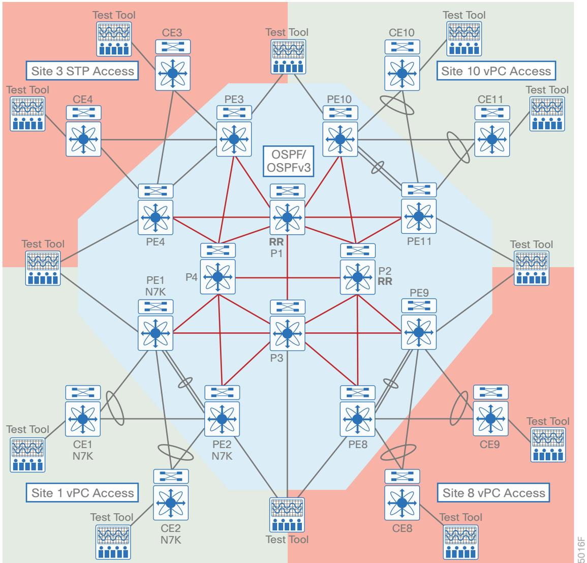
In this diagram, each color represents a different N77 or N7k chassis in which the solid-lined chassis is the default virtual device context (VDC) and the dotted-lined chassis are its non-default VDCs.
