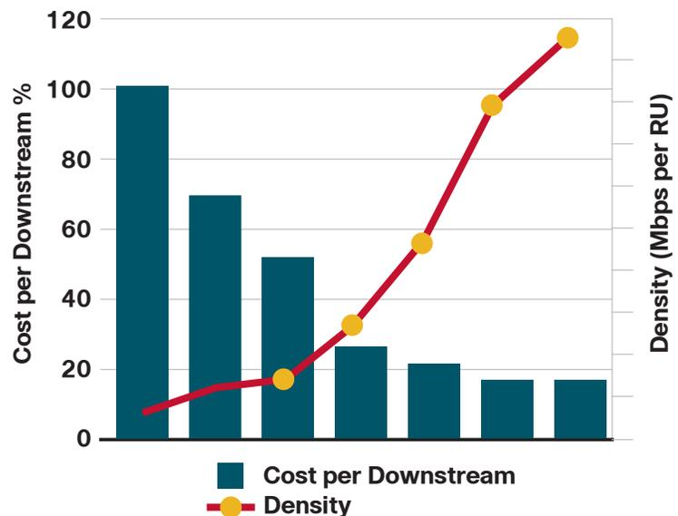
Figure 6. Cisco uBR1000 CMTS Cost and Density Curve
