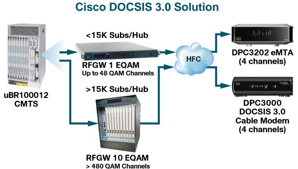
Figure 4. M-CMTS and DOCSIS 3.0 Downstream Channel Bonding
