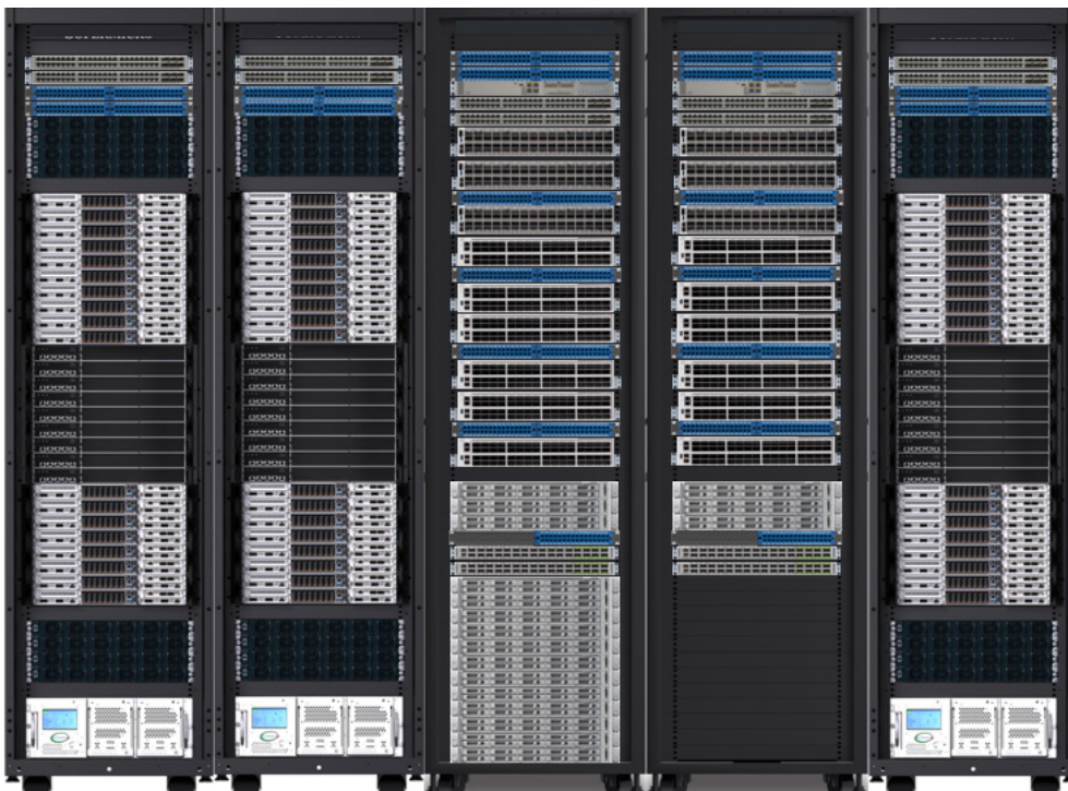
Figure 1. Cisco AI Rack for NVIDIA GB300 NVL72 (Supermicro SRS-GB300-NVL72-M1)
