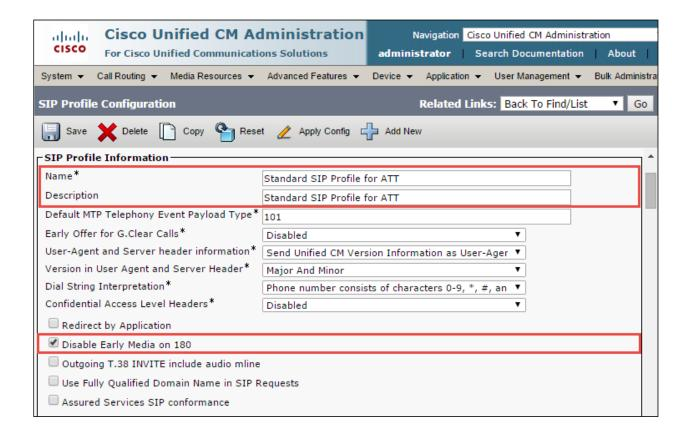
SIP Profile Configuration used by SIP trunk to Cisco UBE (Continued...)
