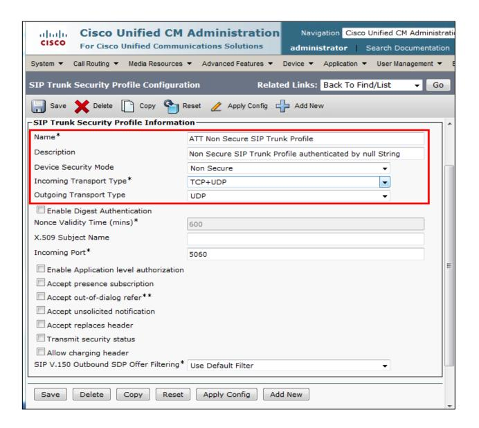
SIP Profile Configuration used by SIP trunk to Cisco UBE
